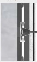
NOTE It is impossible to "short circuit" the DEMARCLIP System when the correct screws are used. Should the installer hit a clip location, they will not be able to 'seat' the screw. They will be forced to move left or right on the track away from the DEMARCLIP.
